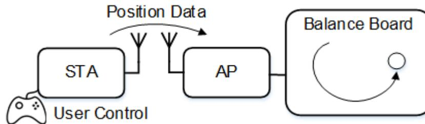
kinematic system comprises of a ball and a balancing board controlled by x and y position servo-motors
