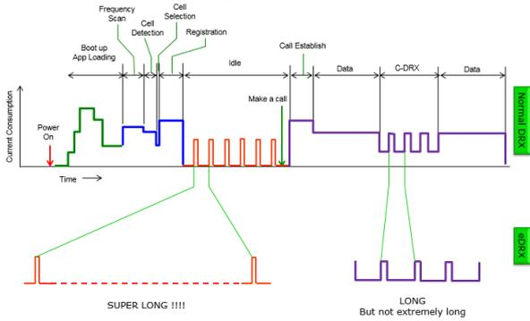
Fig 1. Current consumption with eDRX
