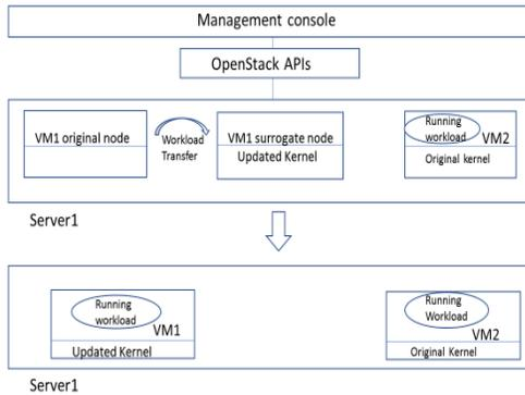
Figure 2: Live update Using OpenStack Technologies
