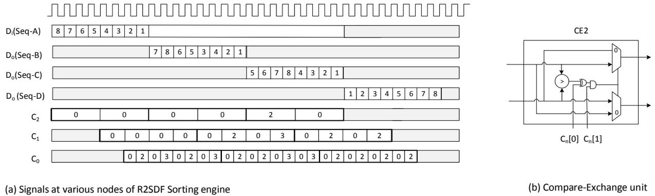
Fig.4 : Waveforms for R2SDF Sorting Engine for N=8
