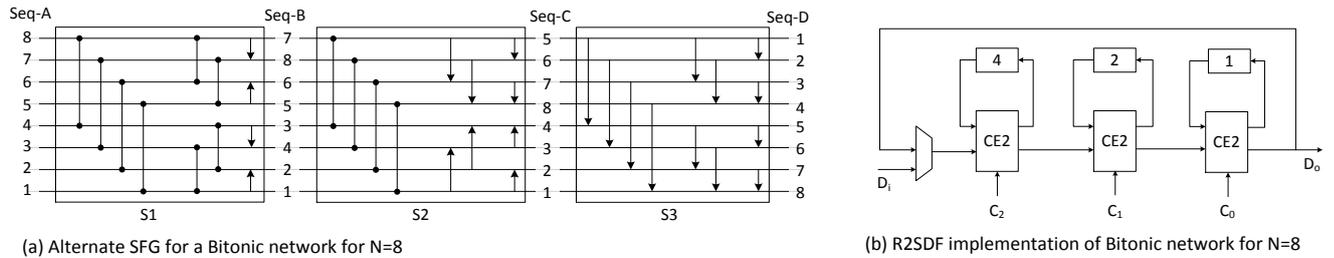
Fig.3 : Mapping a bitonic sorting network to a R2SDF structure for N=8 (with number of iterations = 3)
