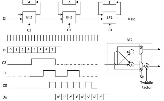
Fig. 2 : R2SDF FFT Structure for N=8
