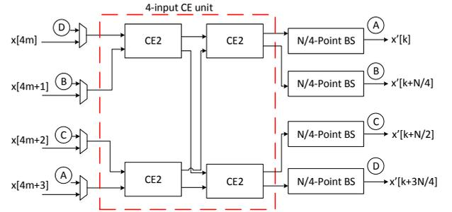
Fig. 6 : 4x Throughput R2SDF Sorting Accelerator
