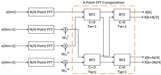
Fig. 5 : 4x Throughput R2SDF FFT Accelerator
