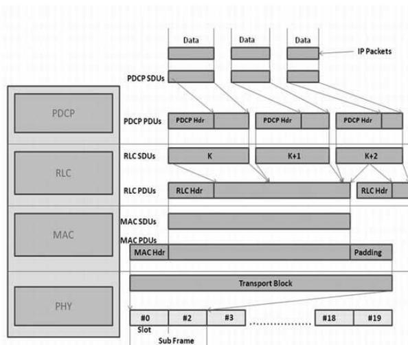
Fig 1. Data Flow through LTE Protocol Stack from [9]
