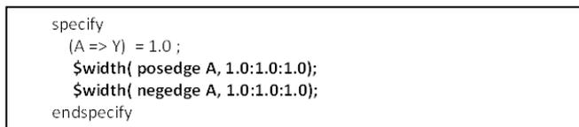
Fig. 8. Minimum pulse width check in verilog
