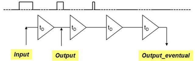
Fig. 3. Pulse width filtering in a delay chain
