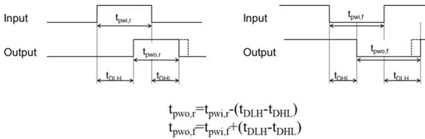
Fig. 2. Pulse width filtering characteristic
