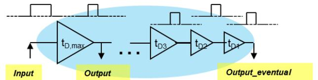
Fig. 5. Delay chain composition
