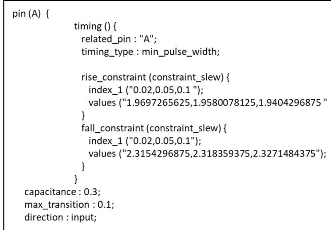
Fig. 7. Minimum pulse width characterization in Liberty timing library
