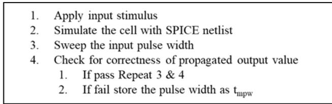
Fig. 6. Characterisation pseudocode for minimum pulse width
