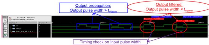
Fig. 18. GLS illustration of a buffer with pulse width filtering modelled
